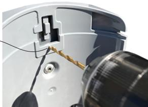
After drilling the hole, run the drill bit up to make the slot
